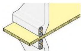
The surface of the FIPRO fire protection boards is to a large extent chemically neutral. Therefore no special adhesives or primers are necessary.
