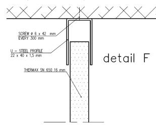
bottom and edge profiles: steel U-profile (22 x 20 x 1.5 mm), or equivalent construction.
