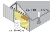
Boards faced, laminated, veneered or coated with HPL may not be exposed to conditions where relative air humidity could drop below 50% or rise above 60%. Air temperatures in stockrooms should not fall below +18°C not rise above +22°C.
